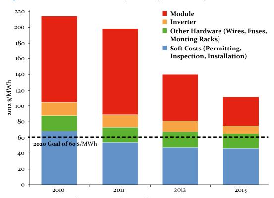
Figure A2: Levelised cost of electricity for Utility-Scale PV Projects
